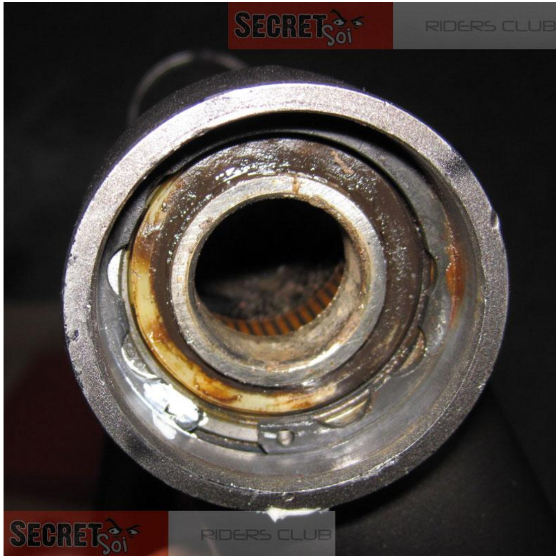
A bit of a mess. The swing-arm was starting to rust and the ball bearing and needle bearing were contaminated.
