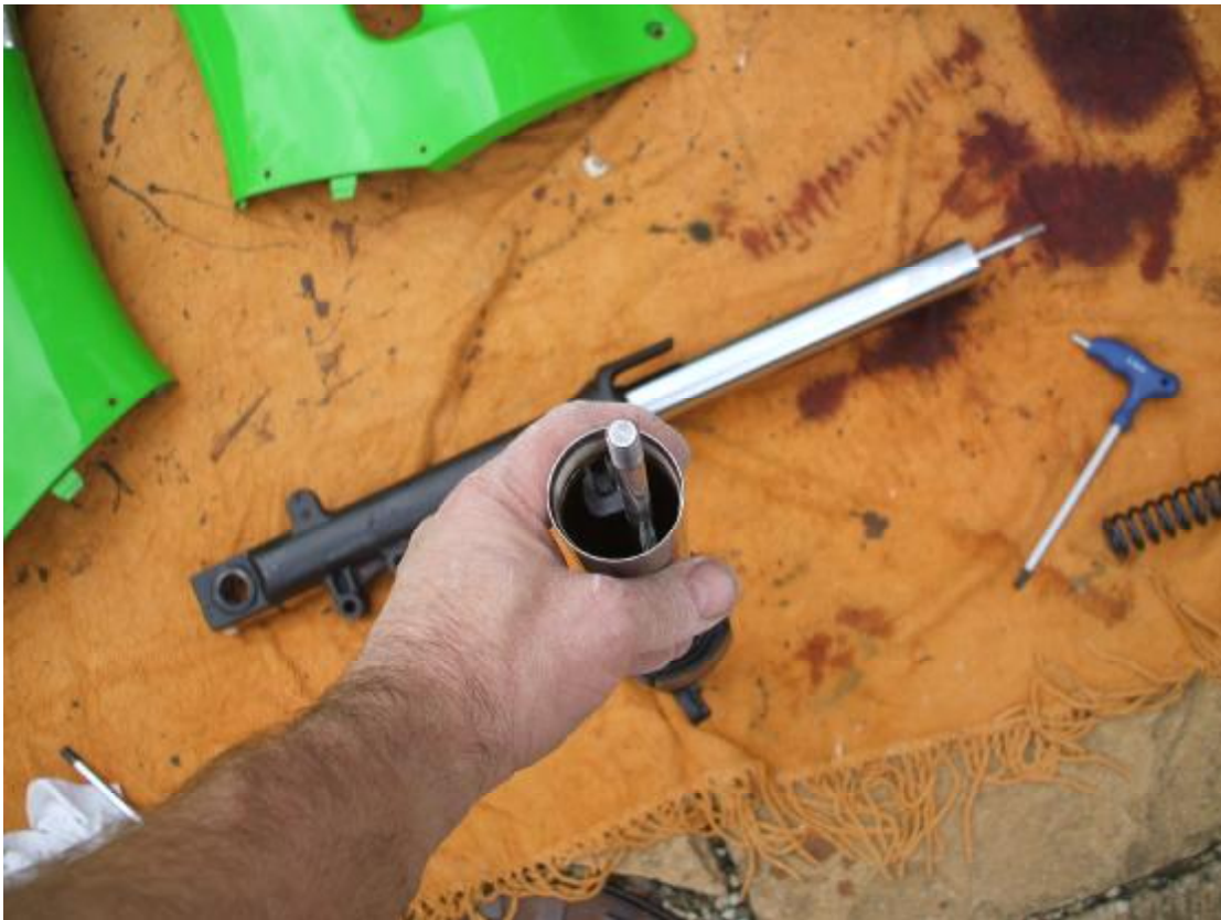
The damper unit, minus spring and fork-top, drops inside the stanchion and slider.
