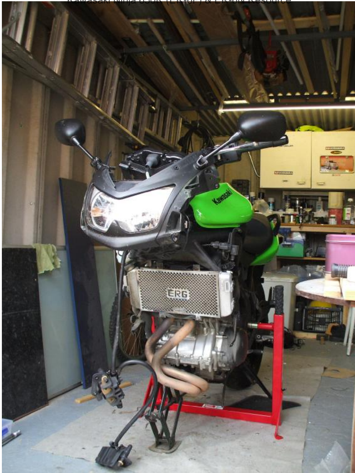
Using an Abby stand I jacked-up the front and removed the front wheel, mudguard and finally, the forks.
