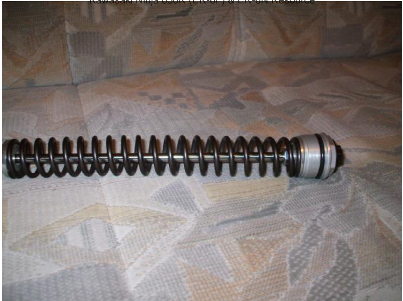
Detail of the spring, damping rod and fork-top.
