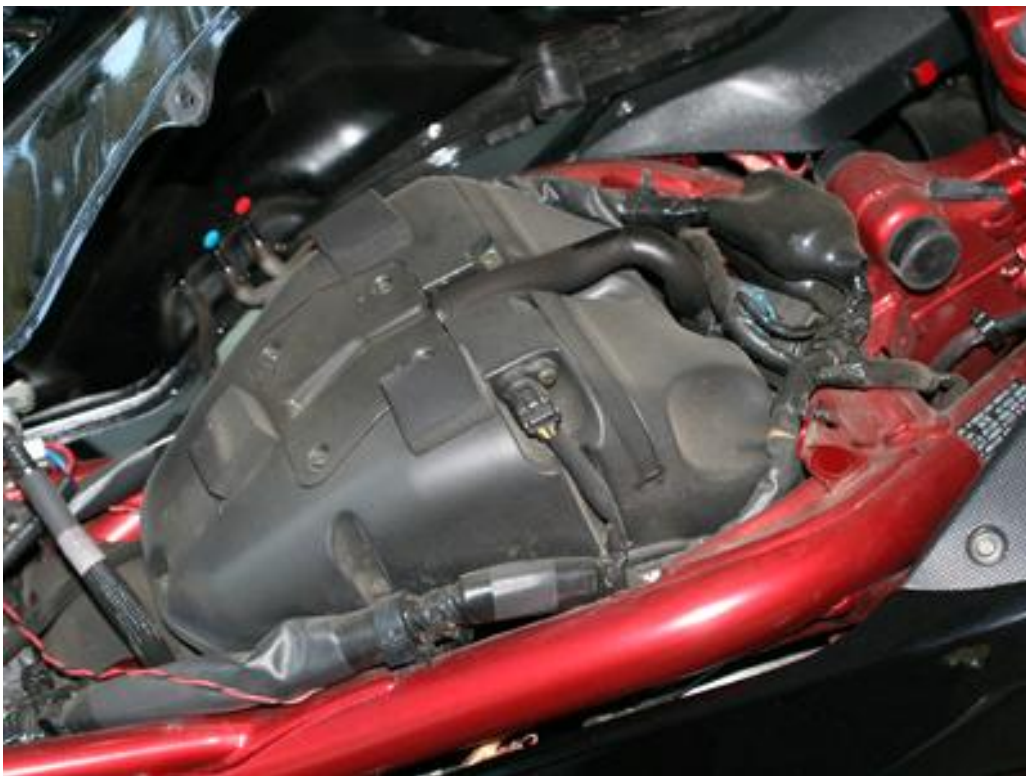
Disconnect the wire harness for the fuel pump.
