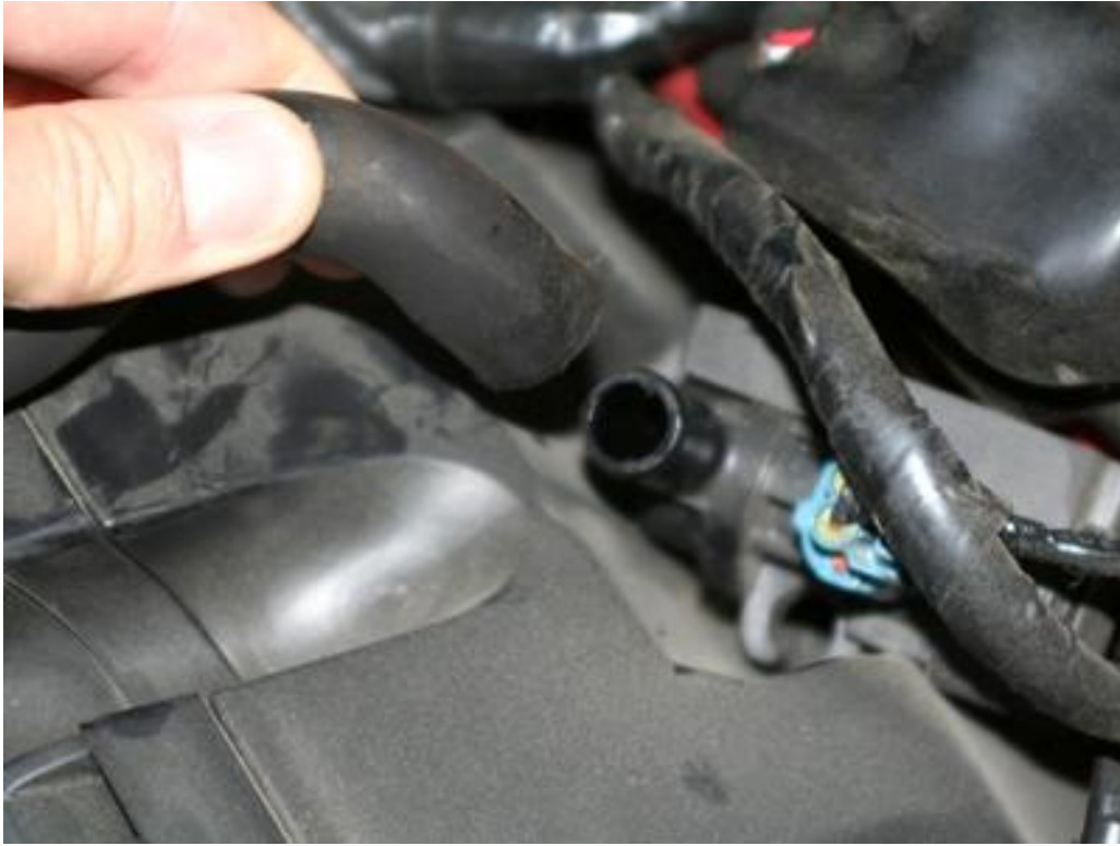
Remove the hose from the PAIR Valve
