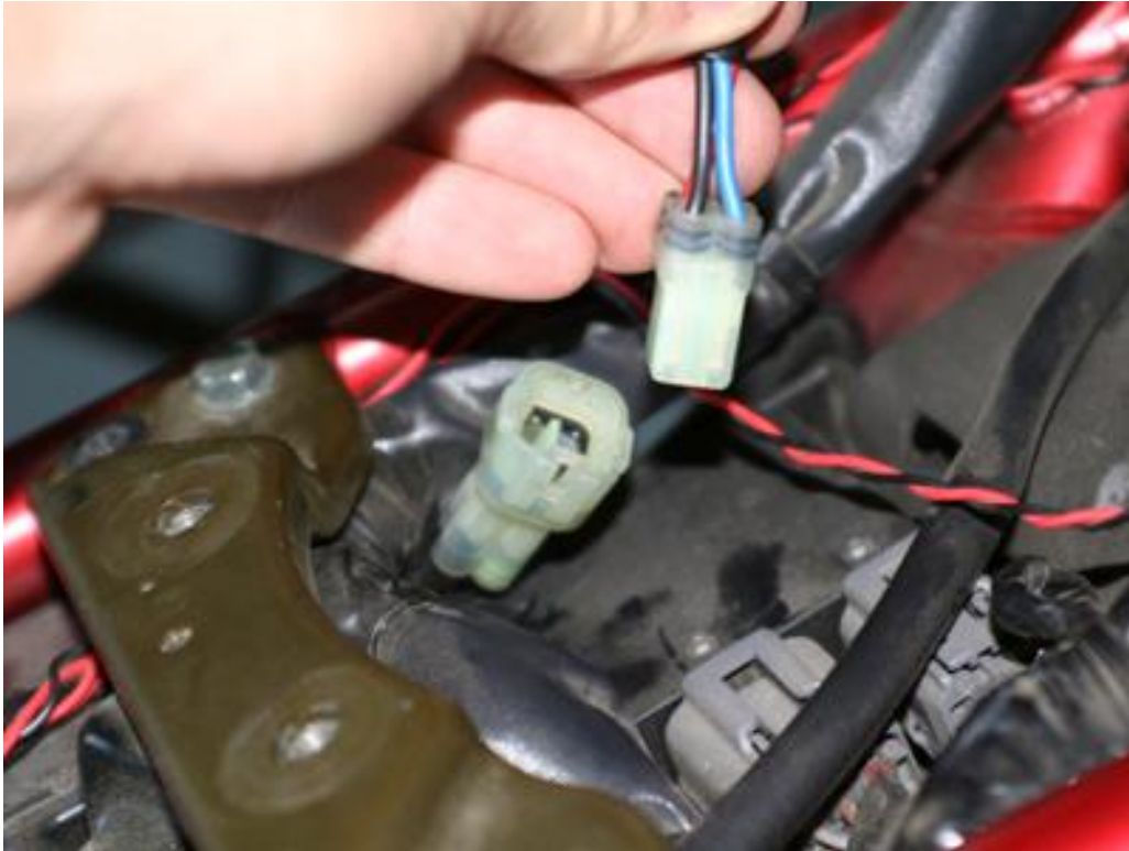
Disconnect the wire harness for the fuel pump.
