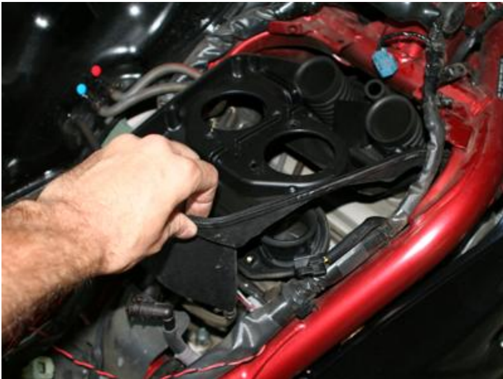
Unbolt the throttle lower with a 5mm socket wrench.
