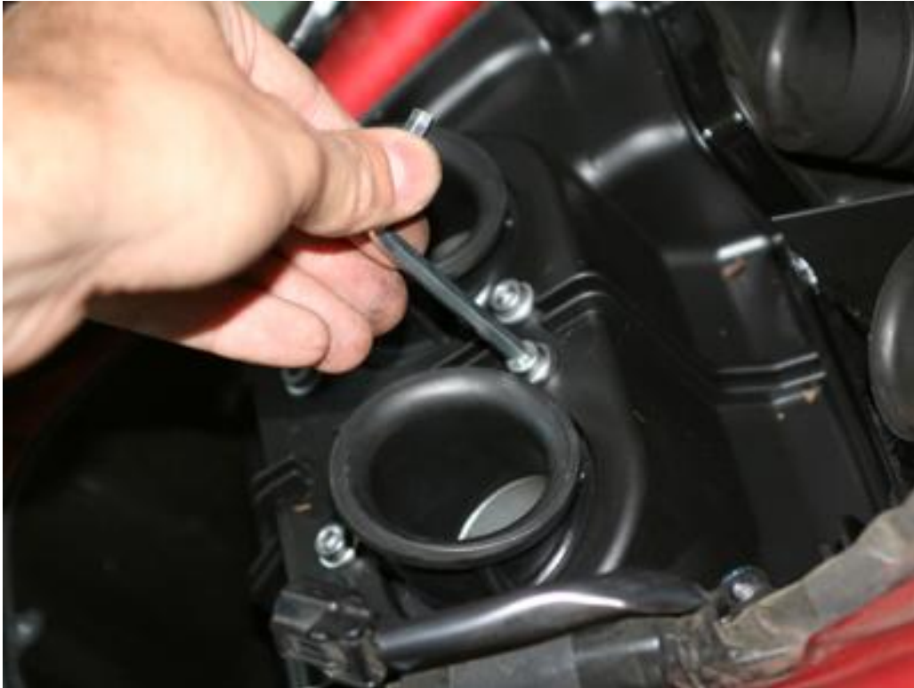
Unbolt the throttle lower with a 5mm socket wrench.
