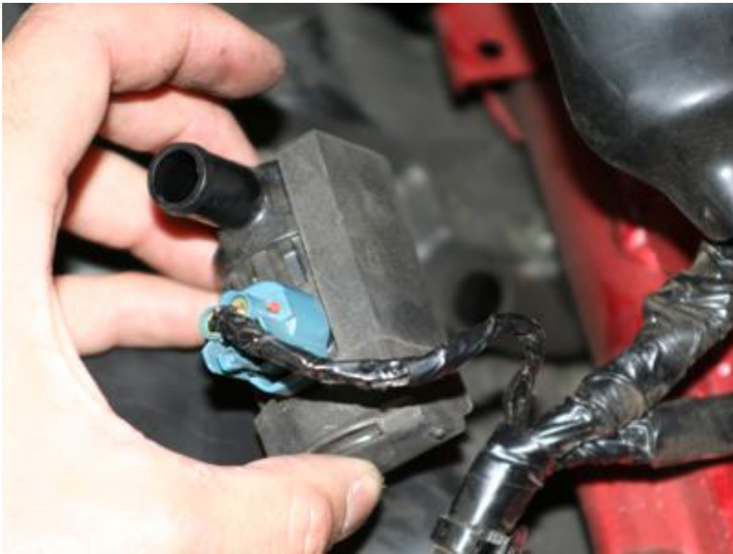
Remove the hose from the PAIR Valve
