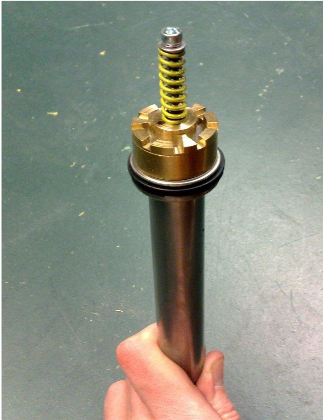
Emulator: - valve sitting on top of the damper rod.
