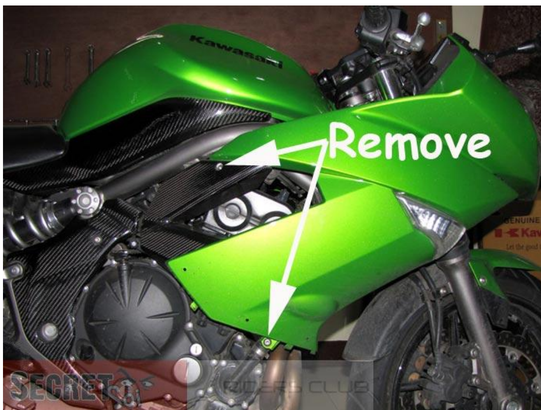
Step 7) Remove the Center Cowlings- Left:
